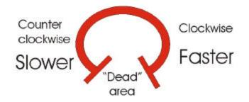
With all pot adjustments, clockwise rotation will increase the cycle speed.
