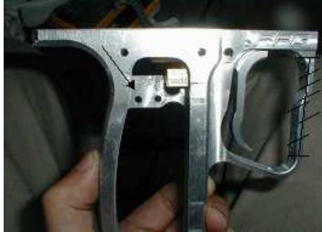
trigger. Get a punch and hammer and punch out the trigger hinge pin and remove the trigger. By removing the front part of the trigger guard, I am gaining access to the part behind the trigger so I can drill a hole straight
