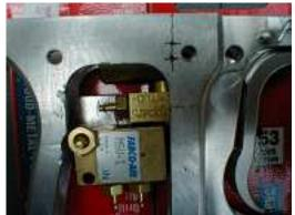
With the frame removed from the marker and the MPA-3 back in the frame in its intended permanent location, eyeball where to drill into the frame so that the setscrews will be on the "flat" part of the MPA-3. When you drill the holes, continue drilling past the frame
