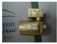
Now, on both sides of the MPA-3, grind it down a little so that it will fit into the frame. Doing it this way is
