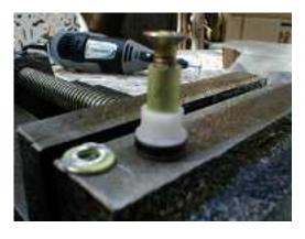
Now it's onto making the piston. Cut the head/disc part off the rivnut and glue the other side to the derlin plunger. I used 2-part epoxy to glue it in. DO NOT loctite the screw into the riv-nut yet.
