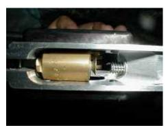
Mounting the Fabco MSV-1 and MPA-3. The Chimera frame is good because you can use the micro switch mount used for the intelli feed to mount the MSV-1. The nut and screw used to mount the MSV-1 is a 6-32 screw and nut. The metal rod to
